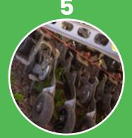
Interrow and intrarow weeding Adjust how close to the crop the FD20 should weed inside the row and start weeding both interrow and intrarow.
